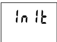
New initialization of logger can occur in switching ON the logger (immediately after displaying of all LCD segments for checking) e.g. after replacement of totally discharged battery for new one. State is indicated by INIT reading. It can be displayed for about 12 s.
