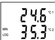
Switched ON logger permanently (with 10 s interval) updates memory of minimum and maximum values. If displaying of MIN/MAX values is selected, minimum measured value is displayed at the LCD lower line (indicated by symbol MIN) and then similarly maximum measured value (indicated by symbol MAX). Upper line always indicates actual temperature. Notice: if alarm is active, no MIN/MAX reading is displayed.
