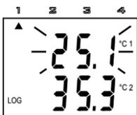
Active alarm is indicated (if display is ON) by blinking of the value of proper quantity on the display and arrow symbol appears at the LCD upper side at the same time. Arrow 1 indicates active alarm for channel 1 temperature, arrow 2 for channel 2 temperature and arrow 4 for temperature difference.
