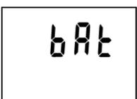
If reading BAT is displayed permanently, battery voltage is low and logger is not possible to switch ON. If logger was switched ON before it, data logging is stopped and logger is switched OFF. Communication with computer can temporarily work. Replace battery as soon as possible!
