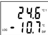
Other measured or calculated values are displayed always after 5 seconds. Instrument now displays channel 1 temperature (°C 1) and temperature difference between channels (lower line "DIF").  $T_{DIF} = T1 - T2$
