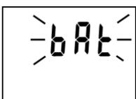
If reading BAT is displayed periodically on LCD upper line (for 1 s with 10 s interval), the end of estimated battery life is coming – however logger functions are not limited. Replace battery as soon as possible!
