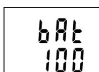
Consequently reading of estimated remaining battery capacity for approximately 2 s is displayed (values 0 to 100%). It is valid if logger is operated at temperature from -5 to +35°C. If logger is operated often outside of the above temperature range battery life can be reduced to 75%, i.e. if displayed remaining battery capacity drops below 25%, it is recommended to replace the battery.
