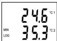
Switched ON logger permanently (with 10 s interval) updates memory of minimum and maximum values of measured values. If displaying of MIN/MAX values is selected, minimum measured value is displayed at the LCD lower line (indicated by symbol MIN) and then similarly maximum measured value (indicated by symbol MAX).
