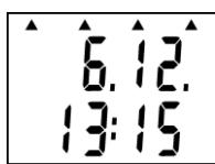
If battery voltage drop occurred since last internal clock setting below critical limit or battery disconnection for longer period than approximately 30 s, after display switch ON (during date and time display) all four arrows appear as warning to check or set it again from the computer. However all logger functions work without limitation.
