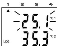
Active alarm is indicated (if display is ON) by blinking of the value of proper quantity on the display and arrow symbol appears at the LCD upper side at the same time. Arrow 1 indicates active alarm for channel 1 temperature, arrow 2 for channel 2 temperature.
