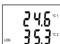
If display is switched ON, actual reading of measured values is displayed - channel 1 temperature (°C 1) at the LCD upper line, channel 2 temperature (°C 2) at the LCD lower line. Symbol LOG indicates data logging in progress – if it blinks, data memory is filled up to more than 90%.
