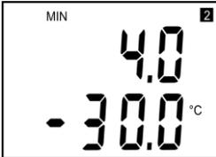
Press button again to display range and type of value for output 2 (symbol „2“). Here it is ambient temperature („°C“), when 4 mA corresponds to -30 °C.
