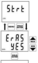
If it is needed to clear the memory before logging start, first it is necessary to select menu item logging START (symbol Strt) and confirm by pressing ENTER key.
