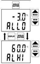
Reading ALLO indicates adjusted lower alarm limit (here air temperature). Set the desired value by means of the arrow keys. Press and hold the arrow key UP to make value increase fast. Press and hold the arrow key DOWN to make value decrease fast. Release the arrow key and press ENTER to confirm new limit
