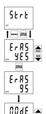
If it is needed to clear the memory before logging start, first it is necessary to select menu item logging START (symbol Strt) and confirm by pressing ENTER key.
