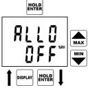
Reading ALHI indicates adjusted upper limit of the same alarm (here air temperature). Set the desired value in the same way as in above lower limit. If needed it is possible to get back to lower limit setting of the same alarm by pressing DISPLAY key. Press ENTER key to confirm new upper limit.
