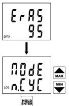
Clearing procedure is in progress. It takes approximately 16 s and the duration is indicated by displaying of already cleared memory in % (digits 0 to 100).
