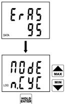
Clearing procedure is in progress. It takes approximately 16 s and the duration is indicated by displaying of already cleared memory in % (digits 0 to 100).
