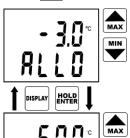
Reading ALLO indicates adjusted lower alarm limit (here air temperature). Set the desired value by means of the arrow keys. Press and hold the arrow key UP to make value increase fast. Press and hold the arrow key DOWN to make value decrease fast. Release the arrow key and press ENTER to confirm new limit.
