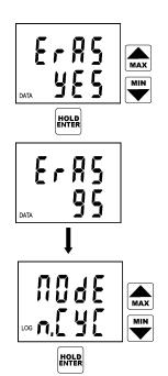
Now instrument offers possibility to clear the memory (ERAS). Default is selection ERAS NO. If clearing of the memory is needed use the arrow keys to select ERAS YES and confirm by pressing ENTER key.
