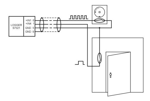
Other possibilities of logger connection to monitored device by means of optional accessory are described at the end of the manual.
