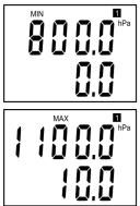
It shows preset value of pressure for voltage output Uout1. Lower LCD line shows voltage value (at V) which is associated to the lowest pressure output (value displayed at upper LCD line). Here 0 V corresponds to 800 hPa.
