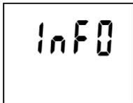
Each pressing of ENTER key causes displaying of service information on software version (upper LCD line) together with instrument configuration on the LCD lower line.
