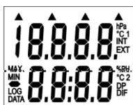
Switch ON the instrument by pressing ON/OFF key. After switching ON the instrument all symbols on the LCD are displayed. If the ON/OFF key is being held pressed, all LCD symbols are displayed till the key is released. In usual operation instrument then starts the measurement mode and actual measured values are displayed. It is possible to switch OFF the instrument anytime and all setting will be saved. Setting will not be saved if battery is disconnected for long than 1 minute.
