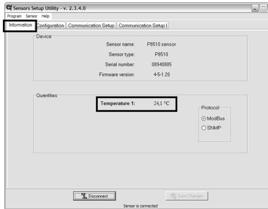
Check measured values. If error value is shown check probes connection and probes configuration on the *Configuration* bookmark (*Channel enable, Probe detection*).
