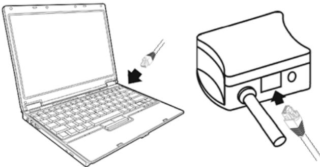
Connect your new P85xx device to PC using crossover Ethernet cable.
