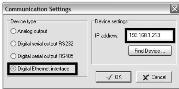
Run T-Sensor software, select device with *Digital Ethernet interface*, insert IP address *192.168.1.213* (factory settings) Click to the *OK* button. If connection to the device fails, use *Find device* button.
