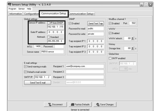
On the *Communication Setup* bookmark configure essential network parameters (*IP address, Netmask* and *Gate IP address*) from step 1.
