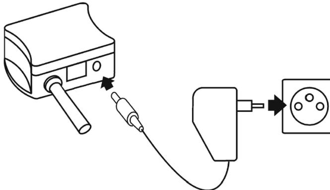
Connect A1825 power supply adapter to P85xx device. You can also use PoE splitter DWLP50 or similar. **Use only power supply adapter recommended by the manufacturer** (5V, 250mA).
