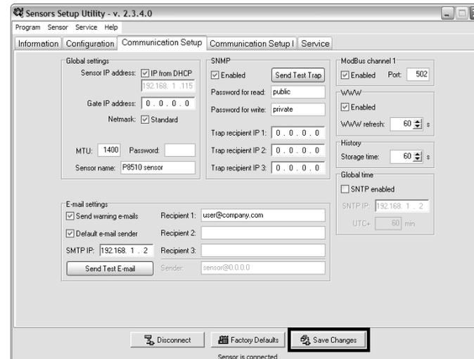
Press *Save Changes* button to save P85xx device configuration. Now the configuration is completed.
